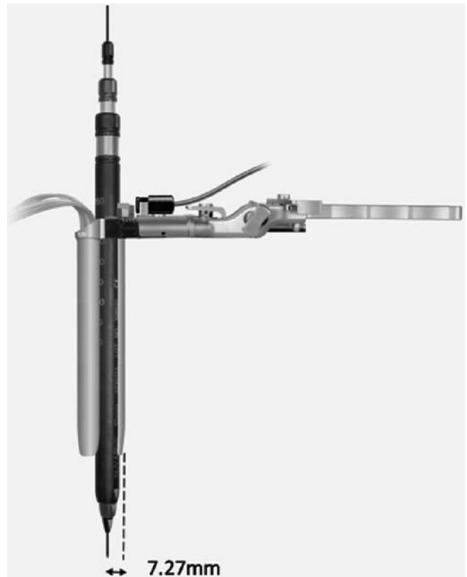
FIGURE 4. Illustration demonstrating the theoretical distance from the guide wire at the center of the MaXcess dilators to the posterior margin of the posterior blade. This distance is the radius of the last dilator (6 mm) plus the width of the posterior blade (1.27 mm) = 7.27 mm. As a measure of neural safety, this number was rounded up to 8 mm as the minimum required distance from the center that the neural structures must be found without having to be retracted during the surgery.
